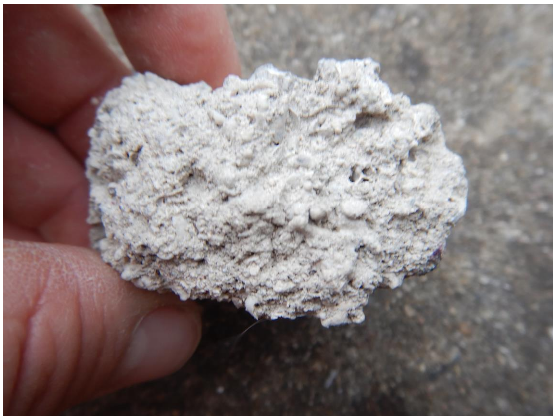
Figure 8. Calcrete cut through by OEM Vibecore from previous project (not Pt Stanvac area) shows cutting potential of Vibecore unit. (A disc shape until chiselled out of the end of the core).
