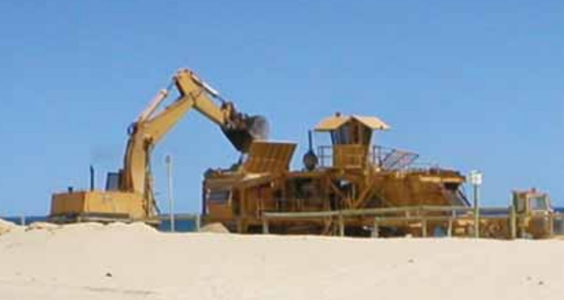
Slurrytrak system in operation at the Dawesville and Mandurah Inlets, Western Australia (CGC Dredging)
